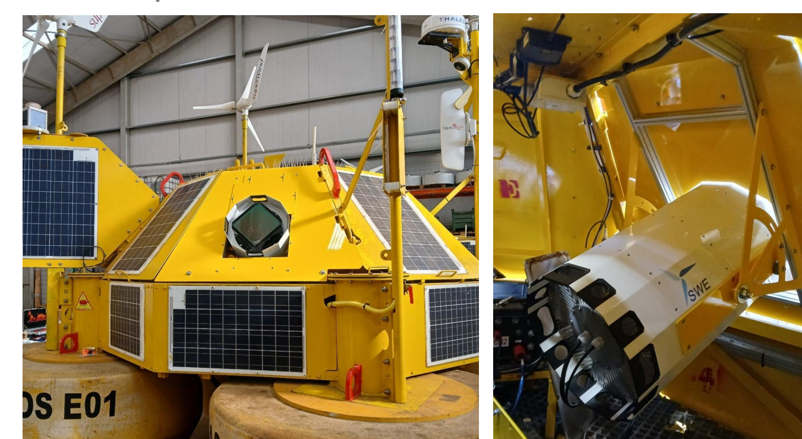
Fig. 2: USTUTT-FSL integrated into the EOLOS FLS200 buoy as part of the LiDAR Modular System (LMS).
