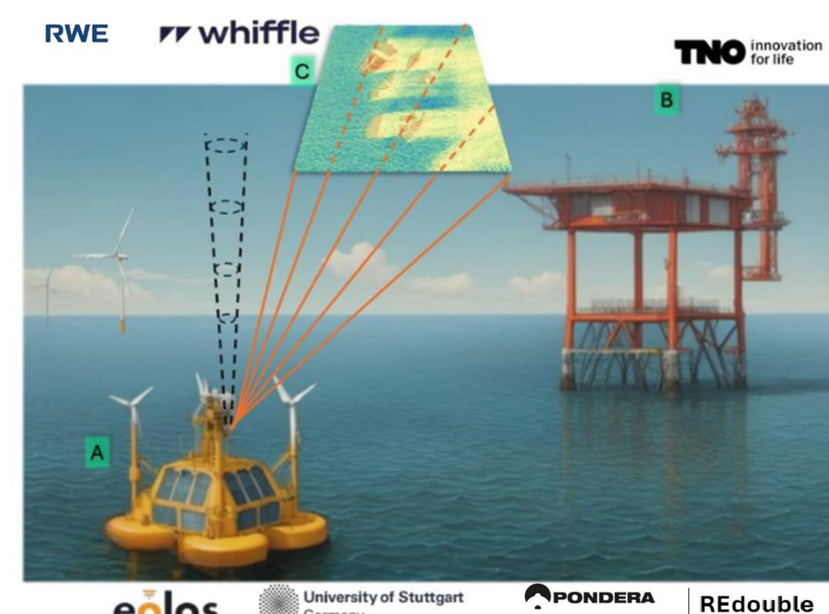
Fig. 3: SSwiFT concept: floating scanning LiDAR measurements, offshore validation and LES.
